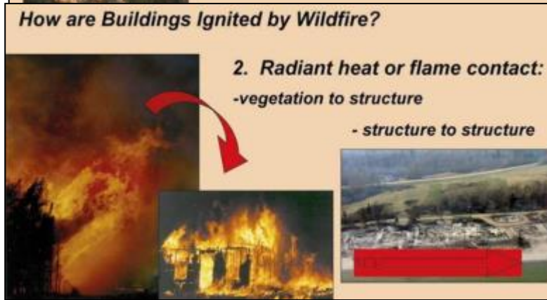
Figure 13. Radiant heat and flame contact allow fire to spread from vegetation to structure or from structure to structure.
