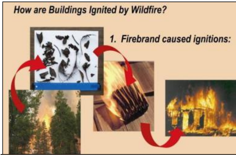
Figure 12. Firebrand caused ignitions: burning embers are carried ahead of the fire front and alight on vulnerable building surfaces.
